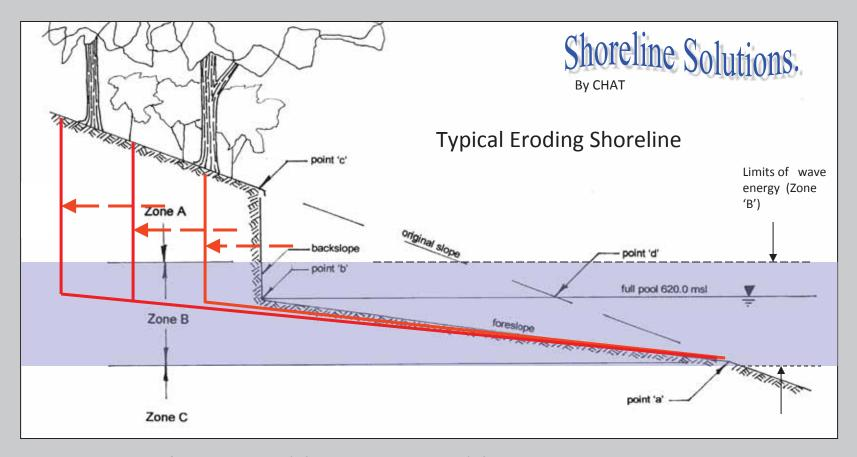
Wave energy is confined to Zone 'B'. The soil in Zone 'B' is taken into suspension by wave energy and is transported to deeper water, where it settles to the bottom and remains indefinitely as sediment.
