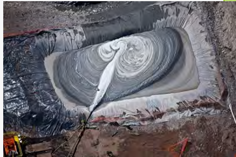
An open pit pond holding slurry from hydraulic fracturing Photo by J. Henry Fair
